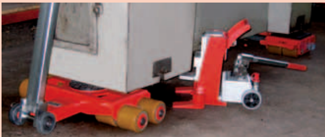
Castors with ball bearings guarantee easy movement
